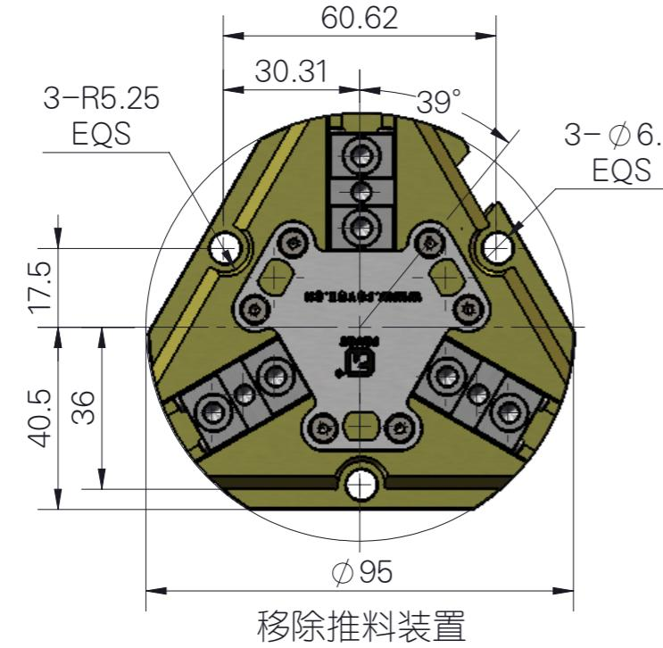
推荐的工件重量 (Recommended workpiece weight) : 5kg
