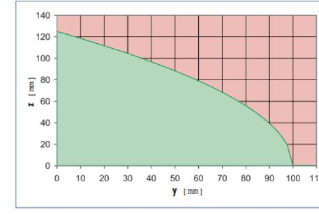
推荐的工件重量 (Recommended workpiece weight) : 4.3kg
